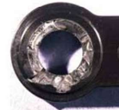
Figure = The failed bracket fracture surfaces exhibited features characteristic of environmental stress cracking (ESC). Source: Thermo Fisher
